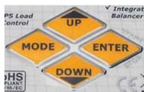
**MODE:** Scrolls between MENUS for MEMORY (Charging), USER SETUP, DATA VIEW, BALANCER
