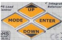
**MODE:** Before Charging/Discharging is started: Scrolls between MENUS for MEMORY (Charging), USER SETUP, DATA VIEW, BALANCER. MODE also selects SOLO and SYNC modes for charging packs greater than 6S
